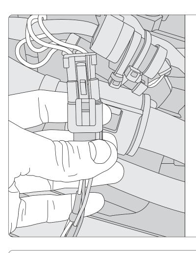
**4)** Plug the HRN-RW07T1 into the corresponding connector on the asset:
